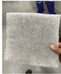
Clean filter Fan CEMs unit 1 &amp; 2
