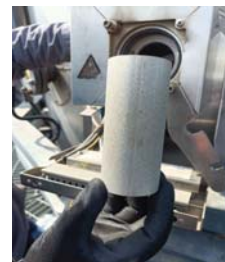
Clean filter probe CEMs unit 1 & 2
